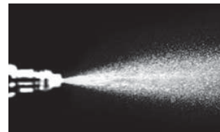
Injector spray pattern after P.i. treatment.
