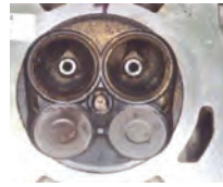
Combustion chamber before P.i. treatment.
