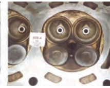
Combustion chamber after P.i. treatment.
